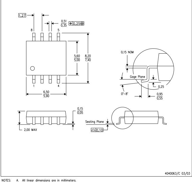
A. All linear dimensions are in millimeters.
